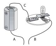
The bulb is not lit. What should be done in order to light the bulb and complete the circuit?
